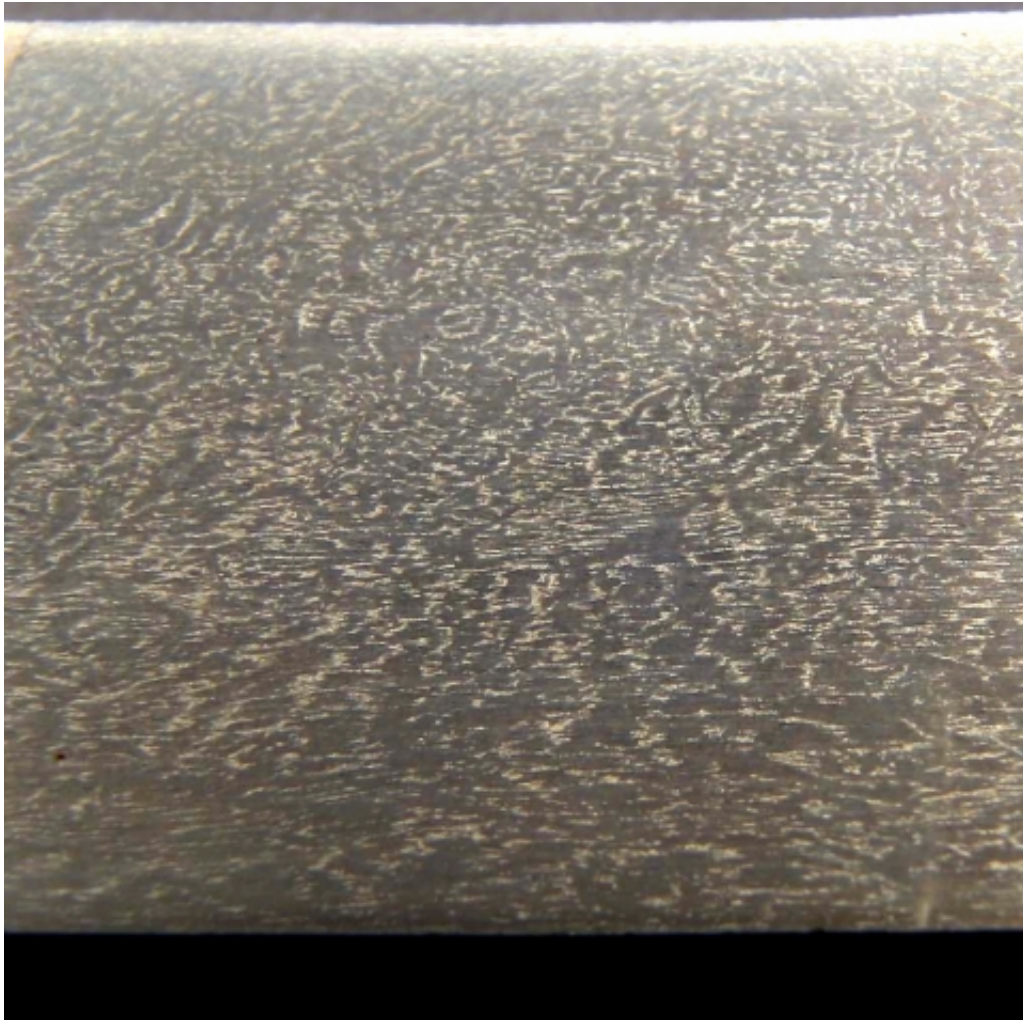
Polished and etched surface of forged crucible steel. The groups of balled up cementite make out the white spots and lines.
