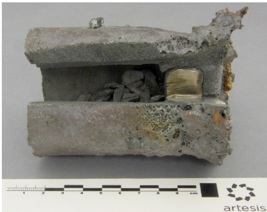
Fig. 4 Crossection of crucible after cooling
