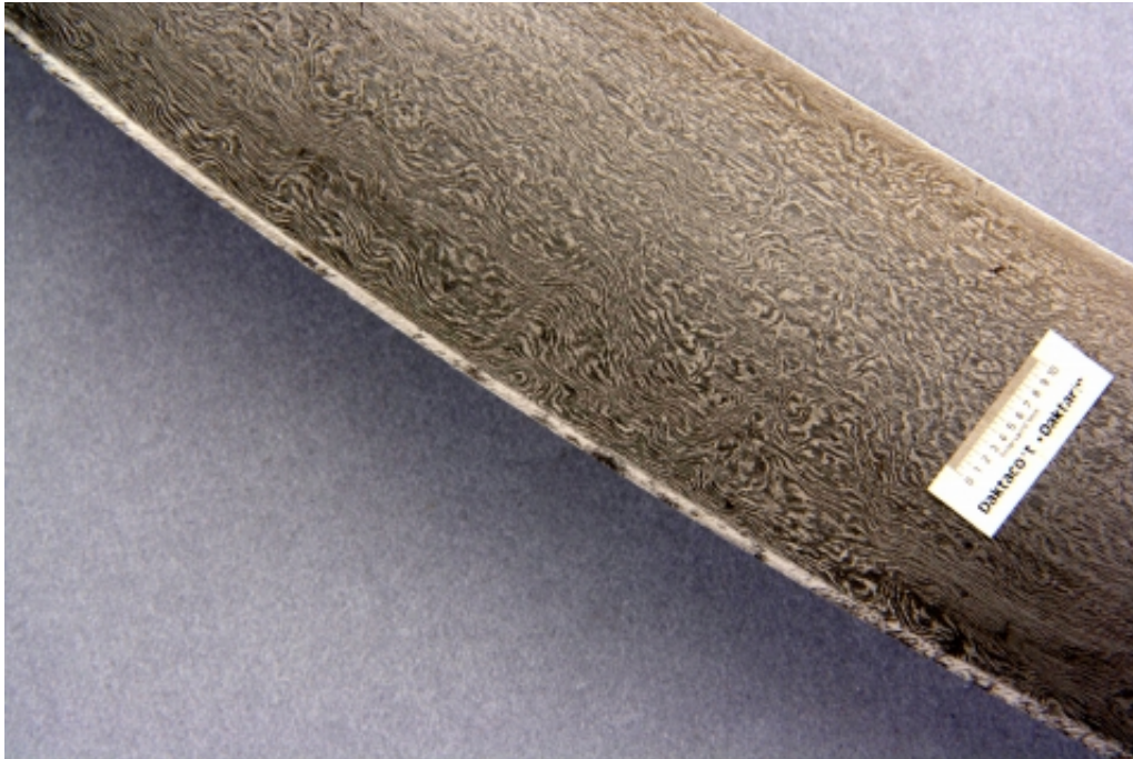
The wavy pattern on the polished and etched surface of the sabre shown in ill.1. This pattern is made out of groups of cementite (white lines) and the steel matrix (black lines)
