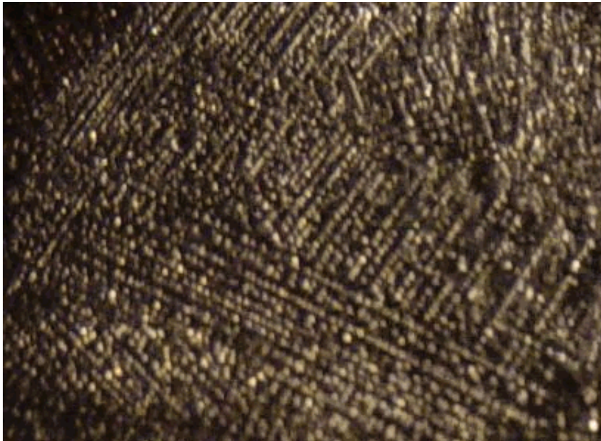
Figure 9. Surface Dendrite displayed on top of ingot, 6X magnification, after removal of glass flux.
